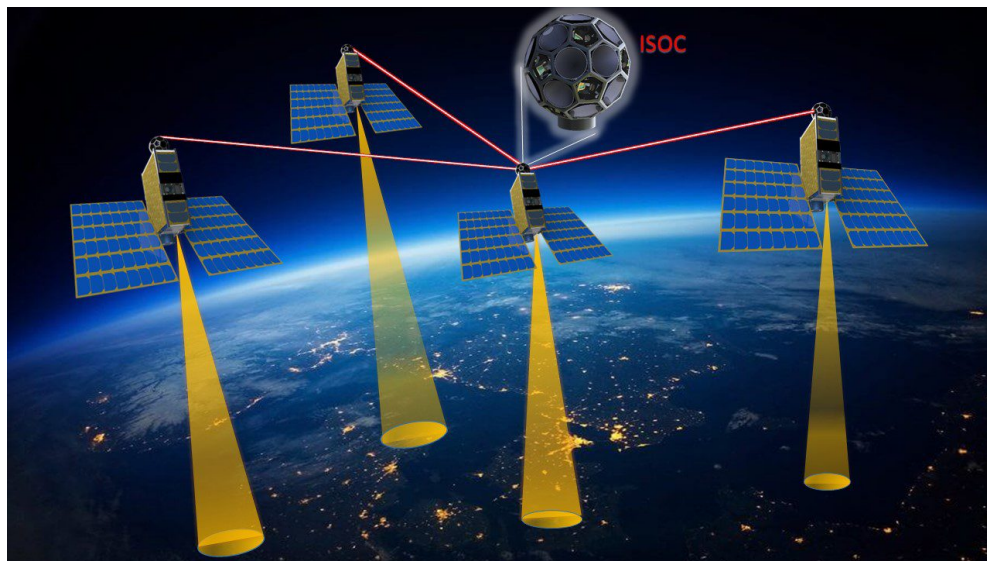
Figure 1. Swarm of CubeSats optically interconnected at gigabit per second speeds via the ISOC. * jose.e.velazco@jpl.nasa.gov
